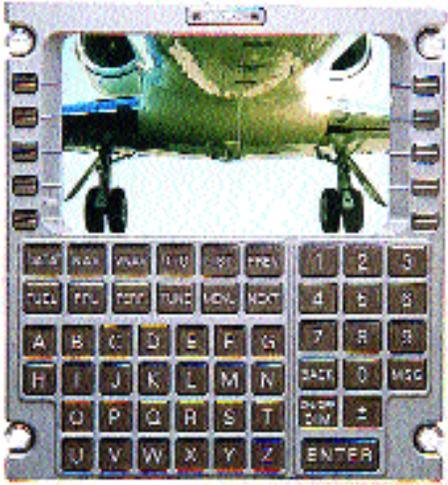
*The crew can inspect the main landing gear condition by utilizing a bottom mounted camera with the display on their CDU in the cockpit.*
